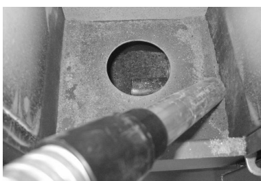
Fig. 31 - Ash tray box cleaning
