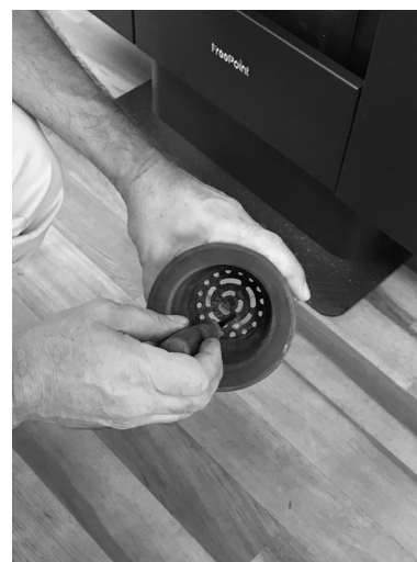
Fig. 30 - Burning pot cleaning
