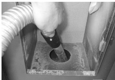
Fig. 32 - Burning pot box cleaning
