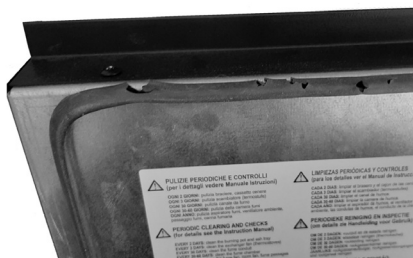
Fig. 24 - deteriorated gasket
