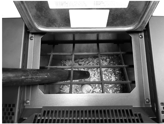
Fig. 34 - Hopper and auger cleaning
