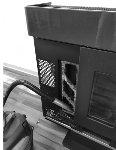
Fig. 38 - Fume chamber cleaning
