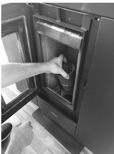
Fig. 28 - Burning pot extraction
